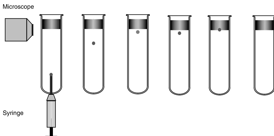
Figure 7.32 Microscopic technique for monitoring coalescence of single droplets at a planar oil–water interface. The time taken for a droplet to merge with the interface is determined microscopically.
